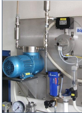
ATEX rated High Vacuum/Multi-Phase Extraction System with LEL sampling system
