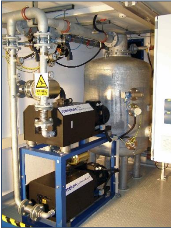
ATEX rated High Vacuum/Multi-Phase Extraction System with LEL sampling system
