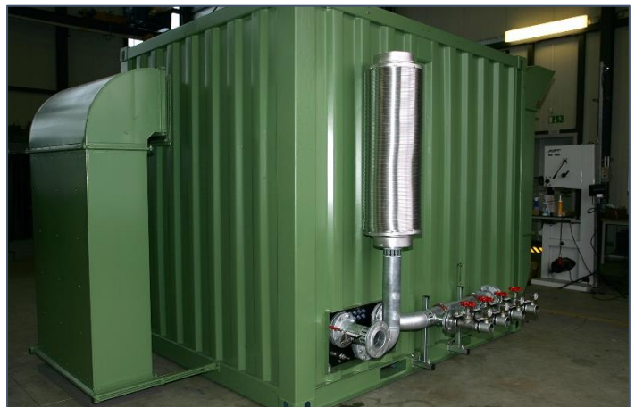
SVE System with acoustic adaptation to achieve 45 dB(A) at site boundary
